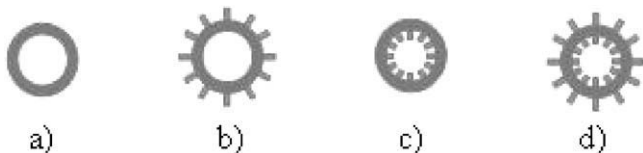
Fig. 1. Possible tube configurations: (a) bare tube, (b) fins on outer surface, (c) fins on inner surface, and (d) fins on both surfaces.
